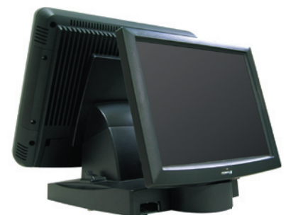
Customer Display Module Optional 12.1" / 15" LCD display unit mounts on rear bracket of ks stand
